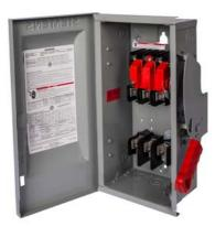
Siemens Low Voltage Circuit Protection Heavy Duty Safety Switch. 3-Pole 3-Wire and negative ground Non-Fused in a type 3R enclosure (outdoor). Rated 600VAC (200A). Special features: photovoltaic rated, 10000 AIC disconnect.
